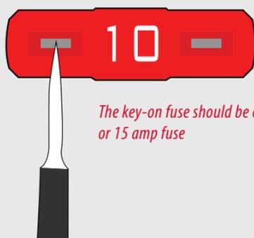
*The key-on fuse should be either a 10 or 15 amp fuse*
