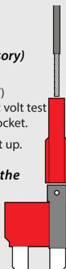
c. Slide the fuse spade over the fuse tap.
