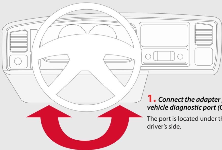
**1. Connect the adapter plug to the vehicle diagnostic port (OBDII).**
